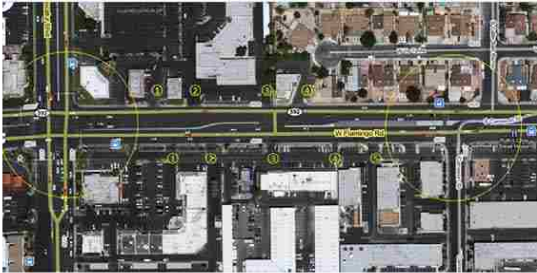
Figure 4-5 Illustration of Driveways and Median Opening
